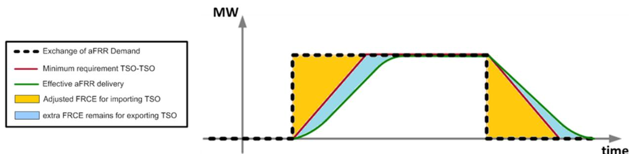
Figure 37: Example of FRCE adjustment volume and TSO-TSO exchange with non-compliant aFRR activation
