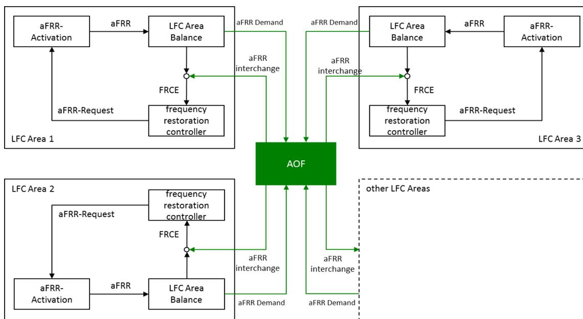
Figure 15: High level scheme of aFRR-Platform
