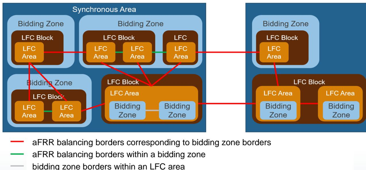
Figure 38: Example LFC structure configuration for participating synchronous areas
