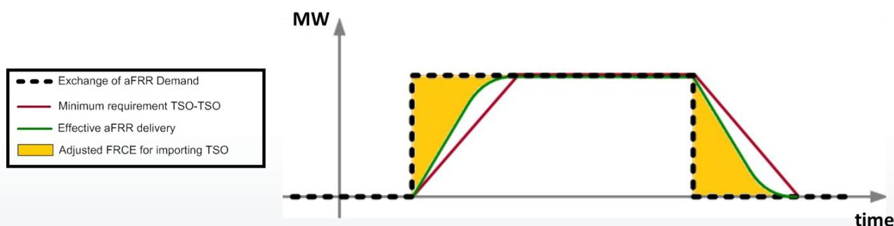
Figure 36: Example for FRCE adjustment volume and TSO-TSO exchange
