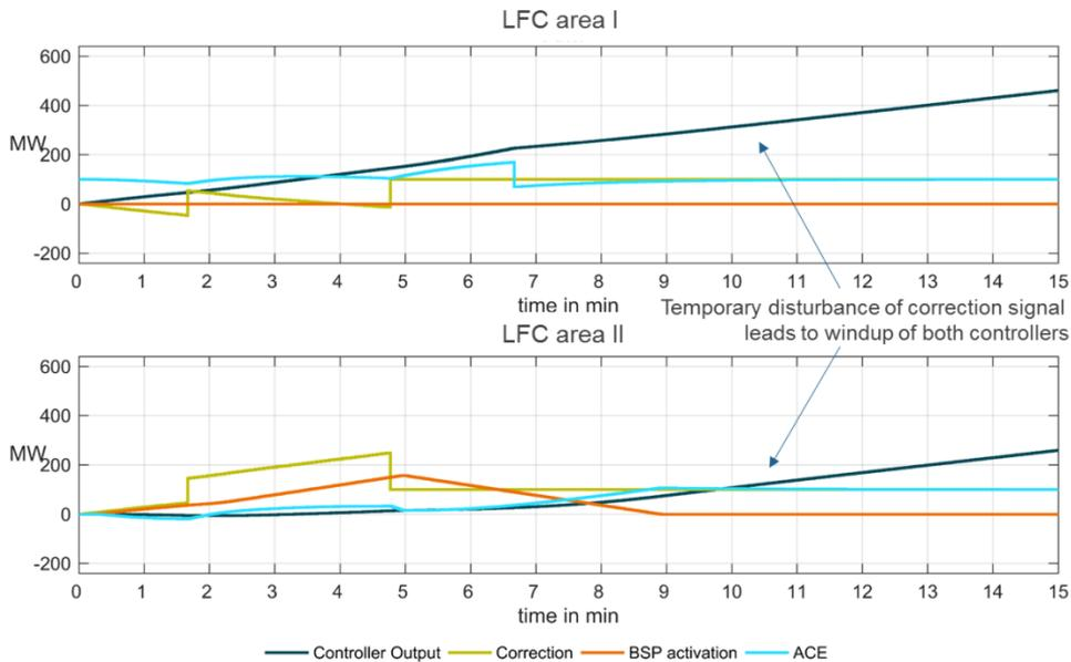
Figure 26: Impact of an IT error in the control request model
