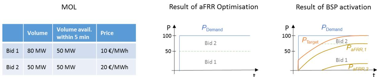
Figure 9: Example of MOL deviations due to dynamic constraints
