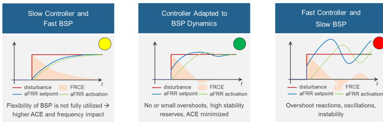
Figure 18: Interaction between BSP behaviour and controller settings
