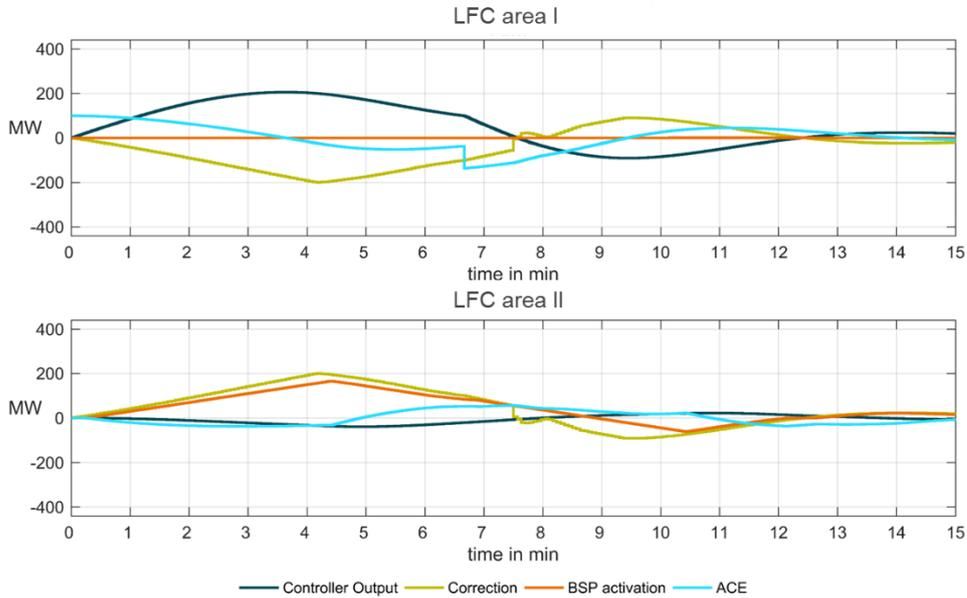
Figure 25: Example of uncoordinated parameterization of LFC with the control request model
